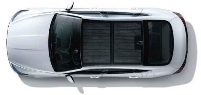
Solar panel roof
