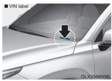
The VIN is also on a plate attached to the top of the dashboard. The number on the plate can easily be seen through the windshield from outside.
