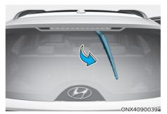
Within 20 seconds after the vehicle ignition is OFF, pull down the wiper lever to MIST position for over 2 seconds until the wiper moves down to the bottom middle part.
