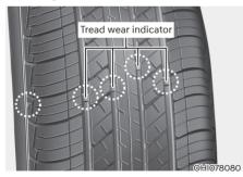
If the tire is worn evenly, a tread wear indicator will appear as a solid band across the tread. This shows there is less than 1/16 inch (1.6mm) of tread left on the tire. Replace the tire when this happens.
