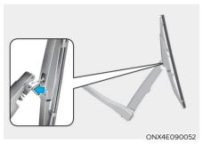
Install the new blade assembly by inserting the center part into the slot in the wiper arm until it clicks into place.
