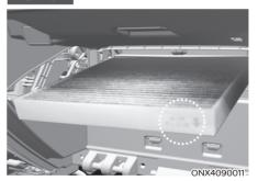
Install a new cabin air filter in the correct direction with the arrow symbol (\*) facing downwards, to prevent noise and improve effectiveness.
