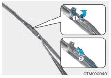
Lift up the wiper blade clip. Then pull down the blade assembly and remove it.
