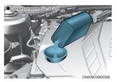
If the oil level is below the L, add enough oil to bring the level to F.
