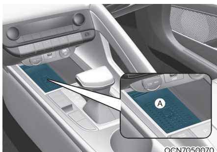
[A] : Charging pad
