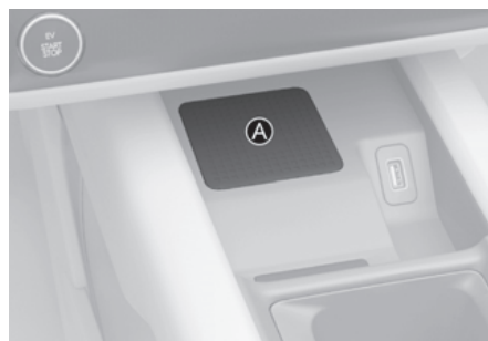
[A] Vehicle authentication pad (Wireless charging pad)
