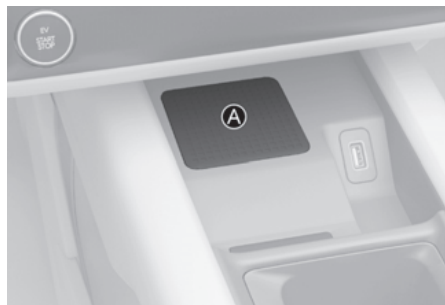
[A] Vehicle authentication pad (Wireless charging pad)
