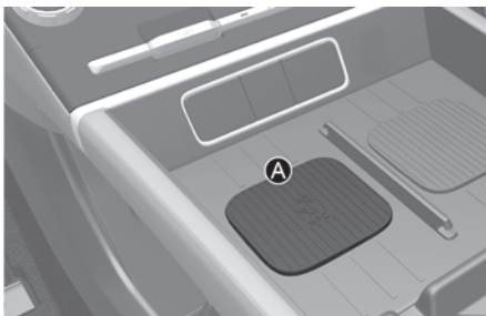
[A] Vehicle authentication pad (Wireless charging pad)
