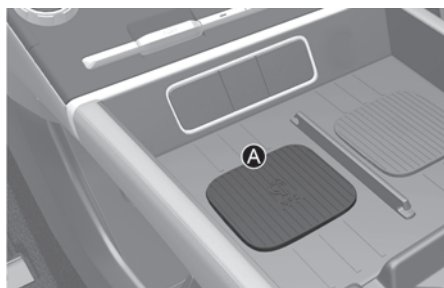
[A] Vehicle authentication pad (wireless charging pad)
